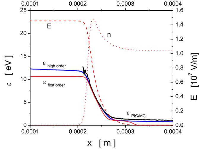
**Figure 3.** Average electron energy in three different models at time 0.7 ns. Profiles of the electric field and the electron number density from the first-order fluid model are also included to indicate the location of the front. Calculations are performed for  $E/n_0$  of 590 Td.
